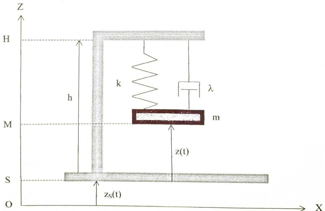
Figure 1 - Sismographe
