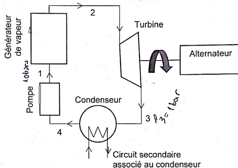
**Figure 6** - Installation motrice
