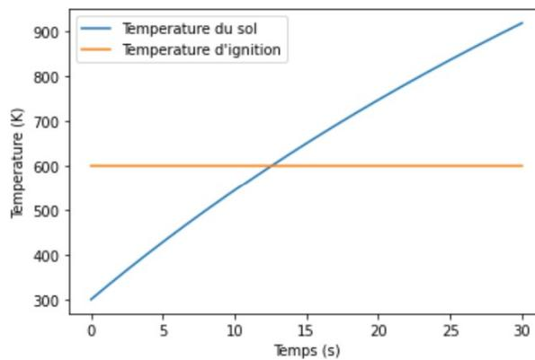
Figure 13: Ignition du sol,  $T_{ig} = 600K$ ,  $\epsilon = 0.9$ ,  $h = 5W/(m^2K)$ ,  $T_0 = 300K$ ,  $C_p = 500J/(kgK)$ ,  $c_{sol} = 0.001J/(kgK)$ ,  $m_{tranche} = 1kg$
